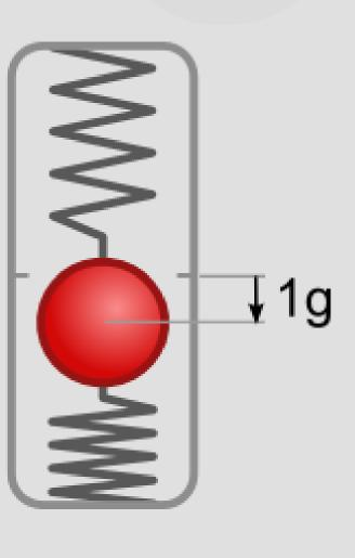
When the phone accelerates, the force from the acceleration displaces a spring.
