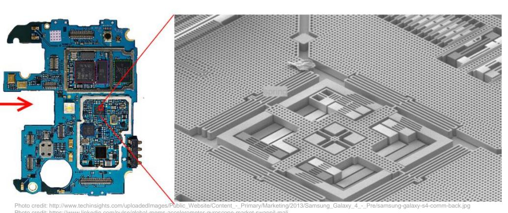
**Inside your phone is a chip with a sensor** the width of a human hair (~80 microns) that measures how your phone accelerates
