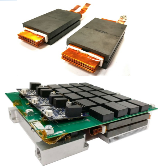
30 kW Composite DC/DC Converter for Drivetrain
